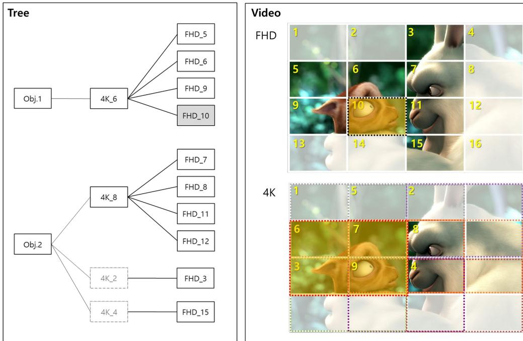
**Figure 7:** Example of tree structure and clip selection for two objects
