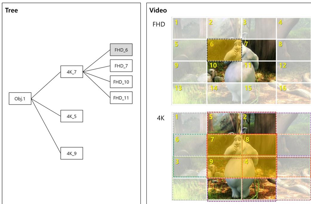
**Figure 6:** Example of tree structure and clip selection for one object
