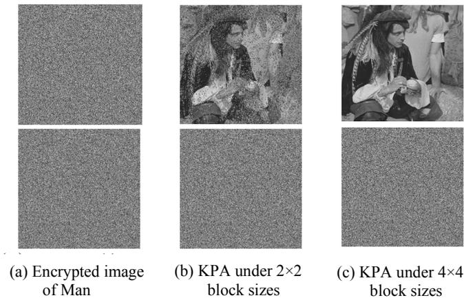
**Figure 8:** (a) Encrypted image of Man. (b) Known-plaintext attack under  $2 \times 2$  block size (c) Known-plaintext attack under  $4 \times 4$  block size. (The first line is the known plaintext attack result of the encrypted image generated by Yin et al. [Yin, Luo and Hong (2014)] and [Liu and Pun (2018)] algorithms, the second line is the known plaintext attack result of the encrypted image generated by the proposed algorithm.)
