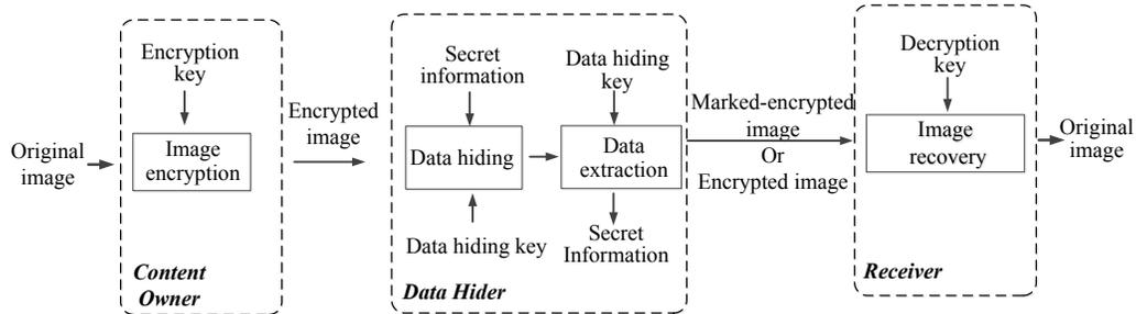
**Figure 1:** The framework of proposed scheme
