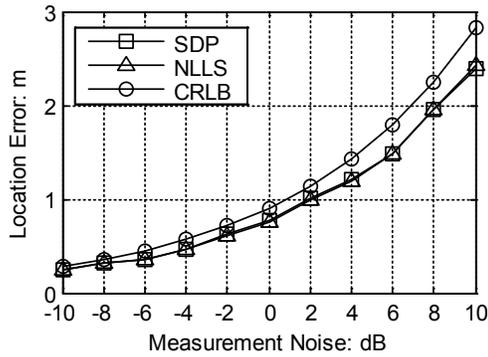
**Figure 1:** The location error when the number of anchor nodes is 5
