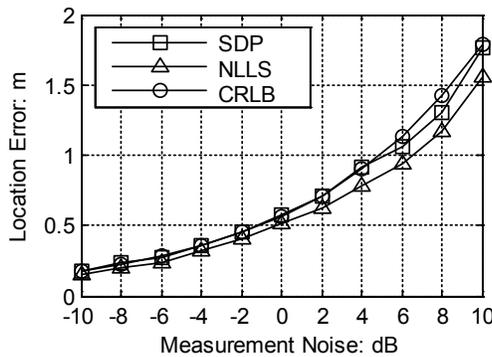
**Figure 3:** The location error when the number of anchor nodes is 9
