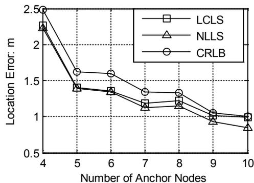
**Figure 6:** The location error when the measurement noise is 5 dB
