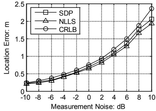
**Figure 2:** The location error when the number of anchor nodes is 7
