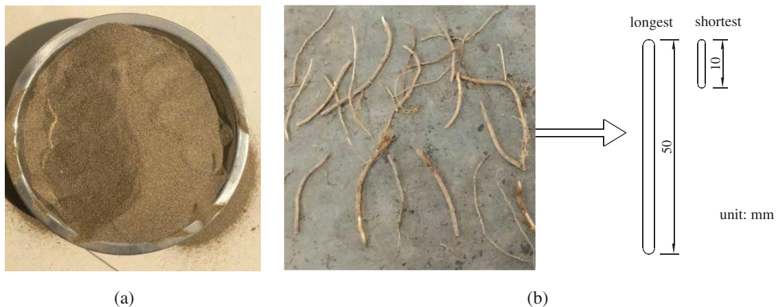
Figure 1: (a) Photograph of Copper slag after grinding and sieving and (b) The roots of Bermuda grass
