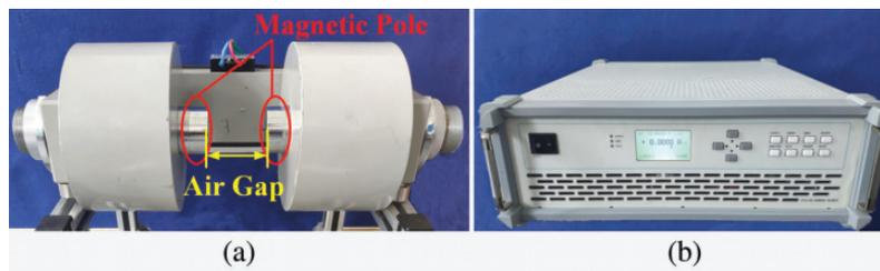
**Figure 3:** Magnetic field generator: (a) Electromagnet, (b) High precision DC excitation source
