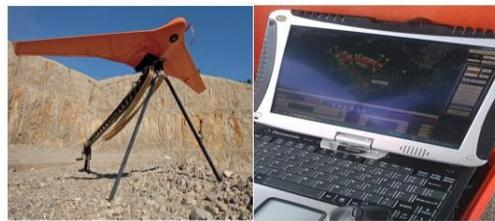
**Figure 1. (a) UAV used for the data collection of the area of interest (b) Software for controlling the UAV.**
