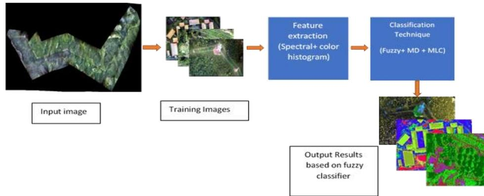
**Figure 2.** Flow Diagram of the UAV-based classification.
