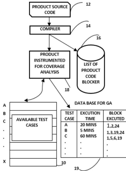
Figure 1. The Genetic Algorithm (GA) based Method to Select a Set of Test Cases (Whitten, 1998)
