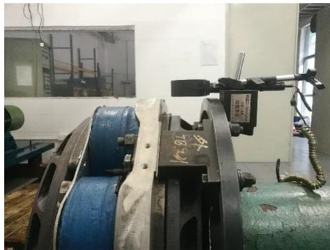
**Figure 7:** Settings of air speed tester for control-type retarder
