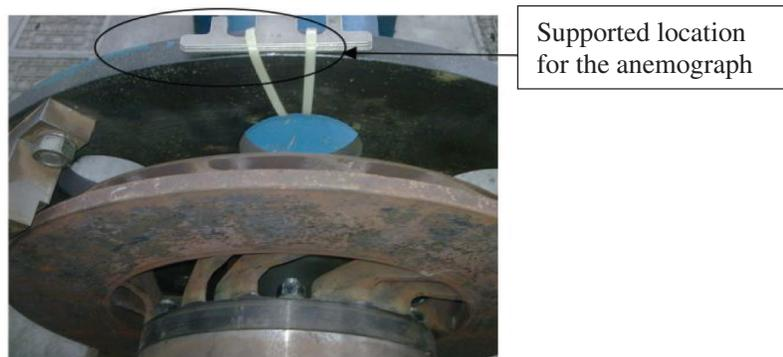
**Figure 9:** Supported position of air speed tester in the control-type retarder's radiator system
