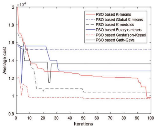
**Figure 6:** Average cost variation vs. iterations number for PSOKM, PSOGlobalKM, PSOPAM, PSOFKM, PSOGK and PSOGG algorithms
