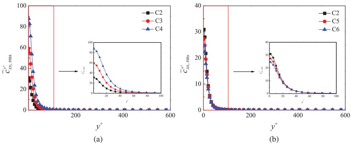
**Figure 6:** Profiles of root-mean-square of  $\bar{c}_{xx}^+$  with  $y^+$ . (a) Different  $We_\tau$  in different cases. (b) Different  $\beta$  in different cases
