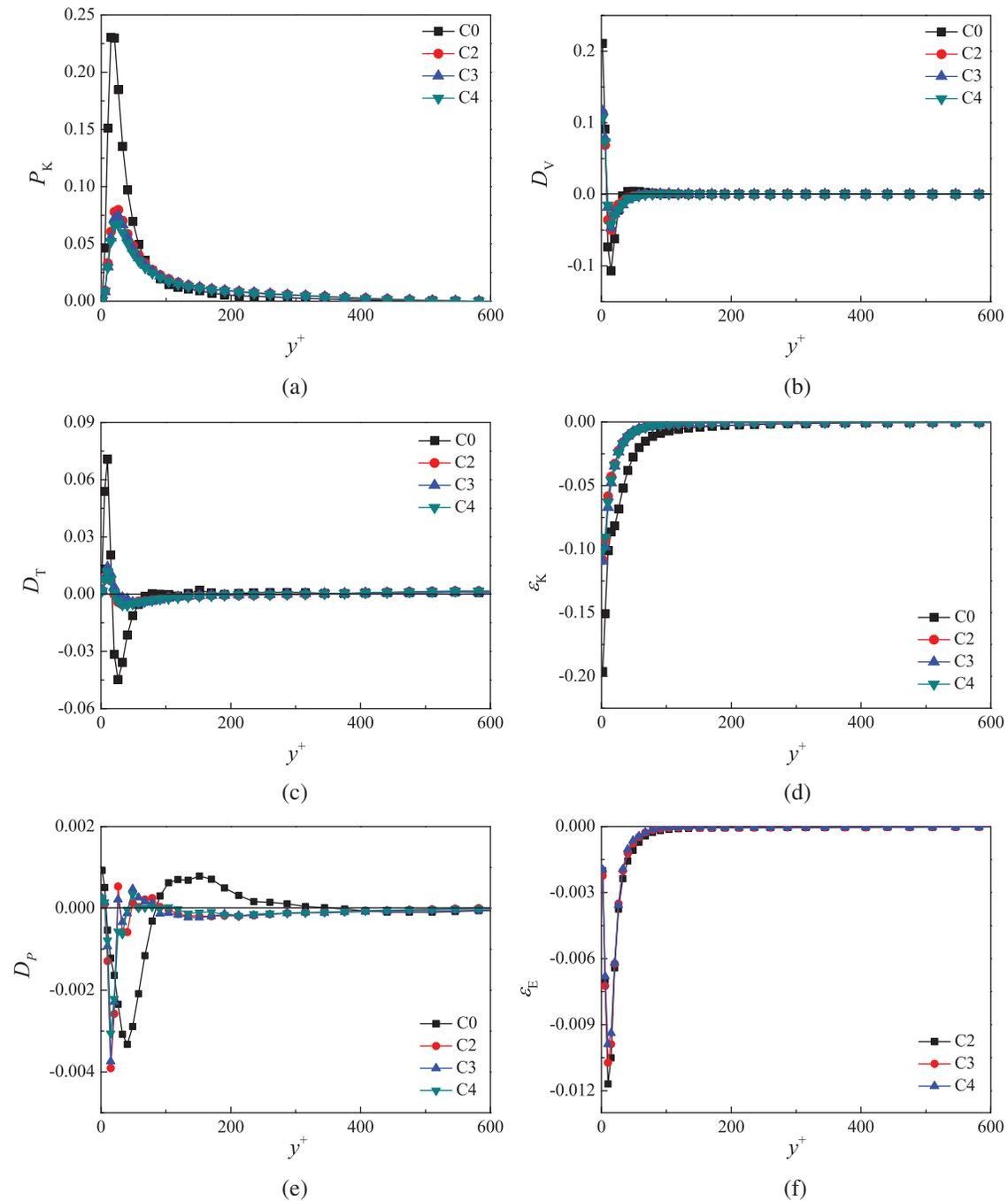
**Figure 9:** Analysis on the balance of turbulent kinetic energy. (a) Production of TKE. (b) Viscous diffusion. (c) Turbulent diffusion. (d) Dissipation of TKE. (e) Pressure diffusion. (f) Elastic dissipation
