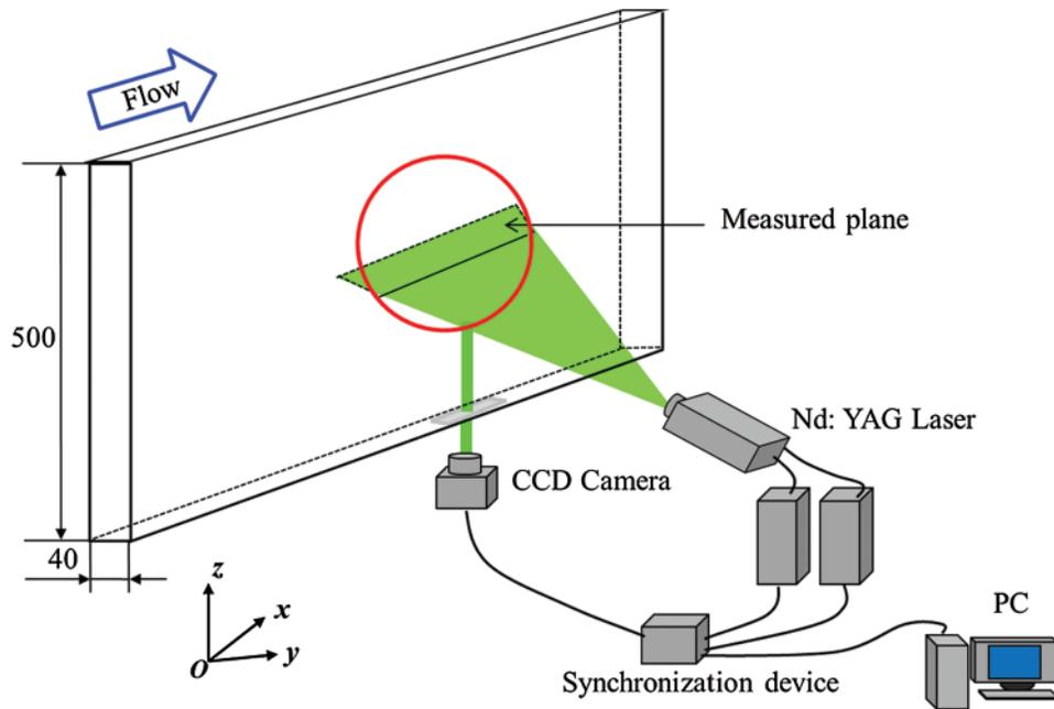
**Figure 3:** Sketch map of particle image velocimetry measurement system (unit:mm)
