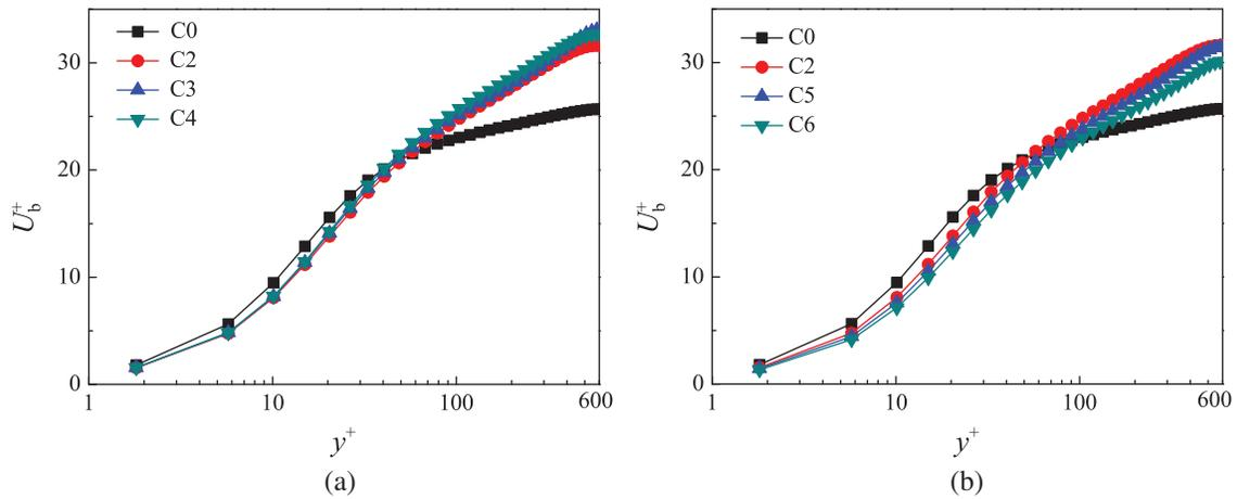
**Figure 5:** Dimensionless streamwise mean velocity profiles. (a) Different  $We_\tau$  in different cases. (b) Different  $\beta$  in different cases
