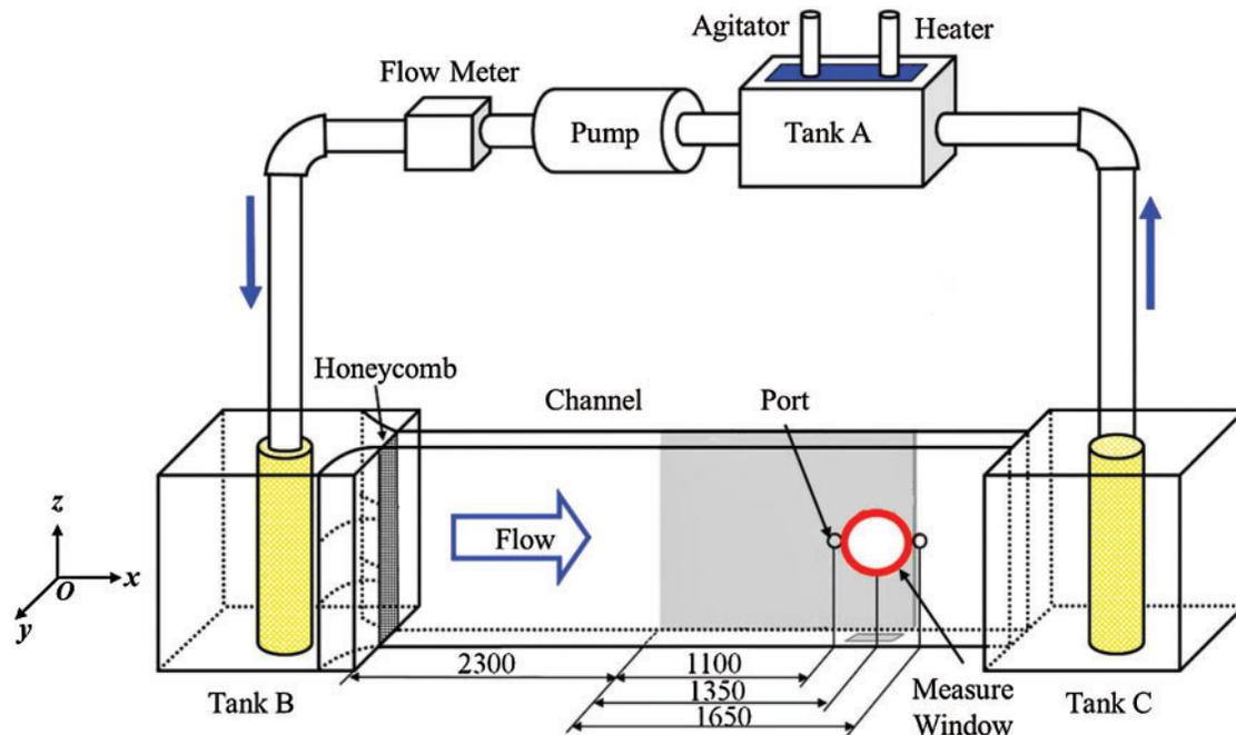
Figure 2: Sketch map of channel flow system (unit:mm)
