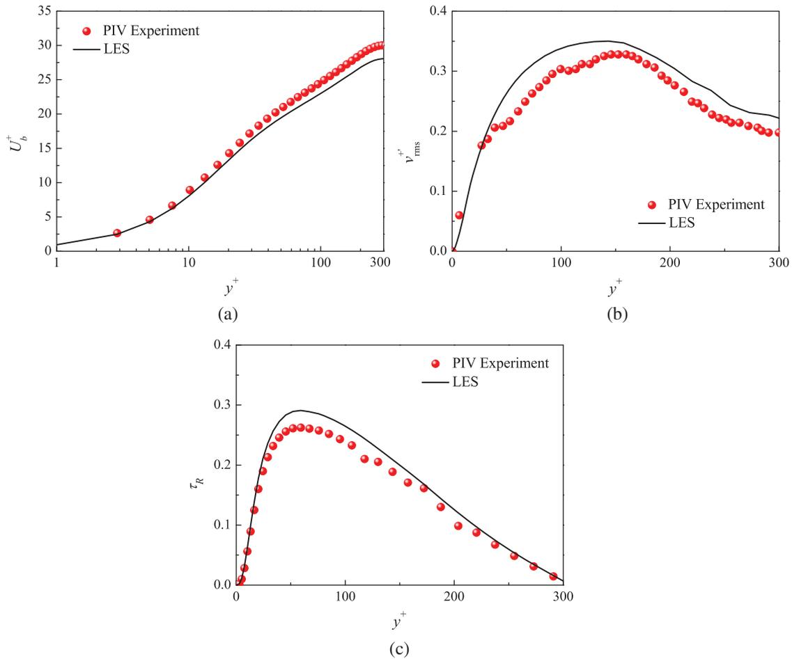
**Figure 4:** Comparison of LES results and PIV results. (a) Streamwise mean velocity. (b) RMS of wall-normal velocity fluctuations. (c) Reynolds shear stress
