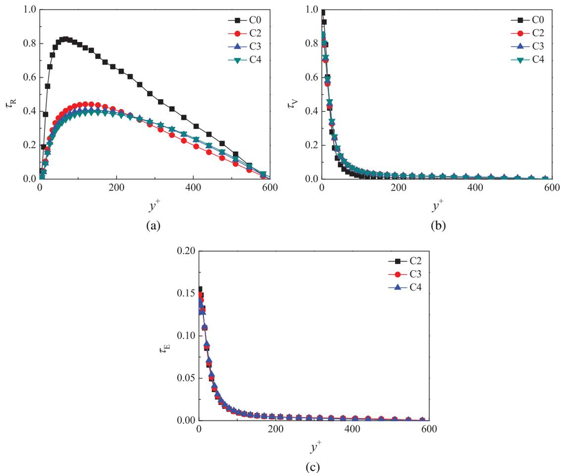
**Figure 8:** Profiles of different shear stresses with  $y^+$ . (a) Reynolds shear stress. (b) Viscous shear stress. (c) Elastic shear stress
