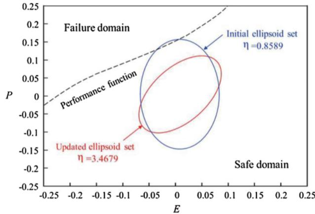
**Figure 8:** The updated ellipsoidal convex model
