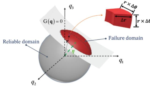
**Figure 3:** A schematic representation of the non-probabilistic reliability assessment
