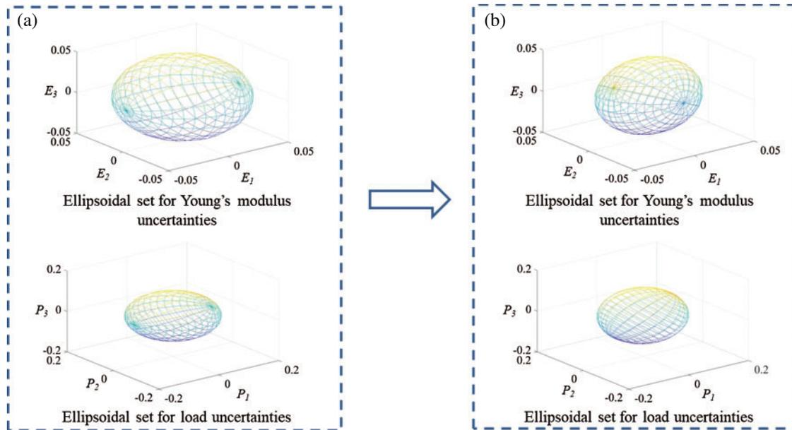
**Figure 13:** The updated multi-ellipsoidal convex model. (a) initial ellipsoid set,  $\eta = 0.9883$ , (b) updated ellipsoid set,  $\eta = 1.1420$
