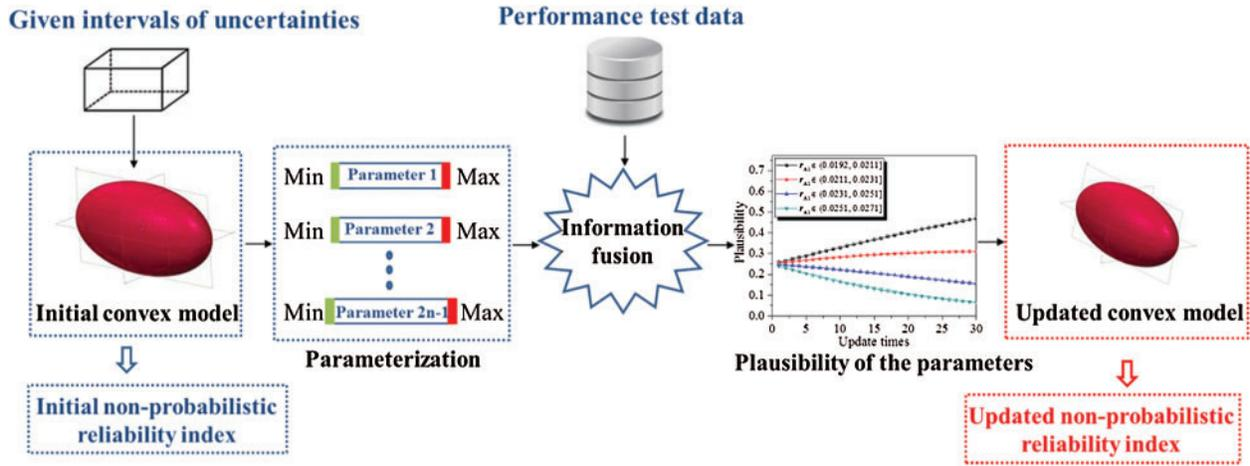
**Figure 1:** Information fusion of prior uncertainty knowledge and subsequent performance test data Jones et al.
