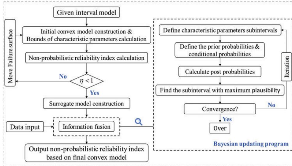
Figure 5: A flow chart of the proposed method
