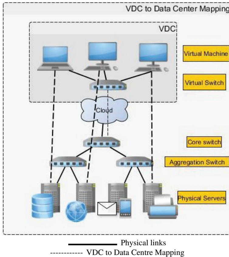
Figure 1 Mapping of VDC request to datacentre.
