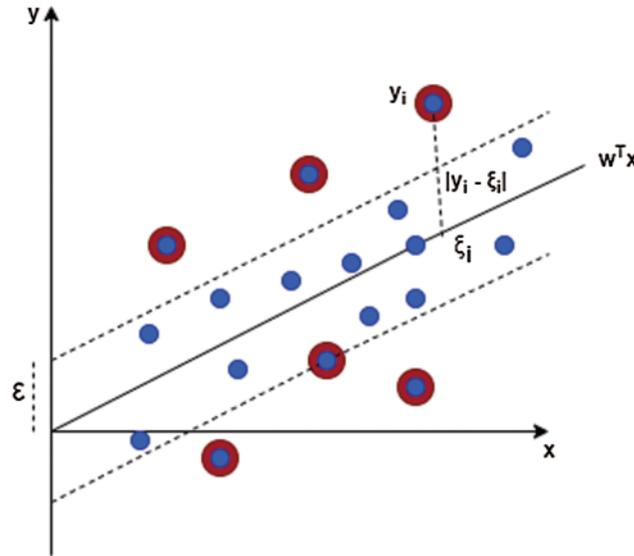
**Figure 2:** Support vector machine regression [37]
