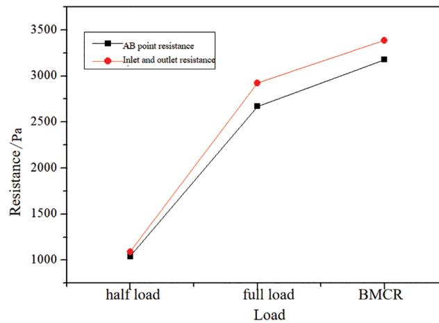
**Figure 2:** Statistics of the global simulation of the static pressure difference
