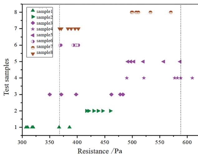
**Figure 5:** Distribution of the resistance of the shell of the bag filter
