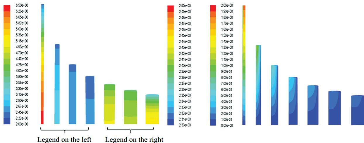
Figure 8: Plots of the static pressure and velocity of the filter bag
