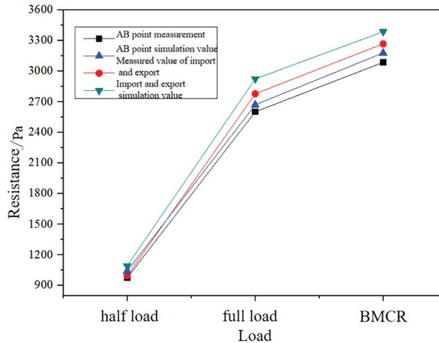
Figure 6: Statistics of the global simulation of the resistance of the bag filter and the measured value
