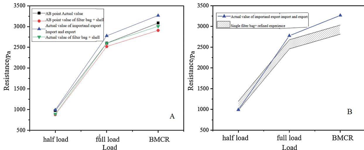
Figure 7: Statistics of the local simulation of the resistance of the bag filter and the measured value
