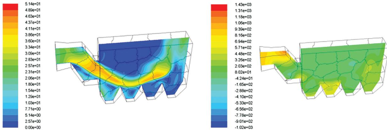
**Figure 4:** Plots of the shell velocity and static pressure at the BMCR point
