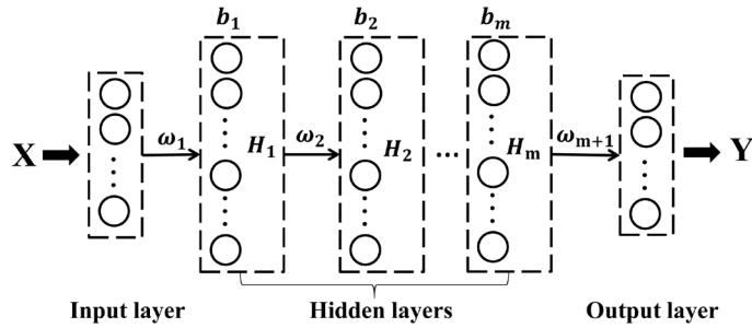
**Figure 3:** The network structure of the deep learning model
