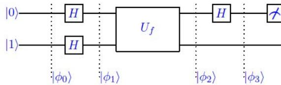
**Figure 4:** Quantumn Circuit for Deutsch algorithm
