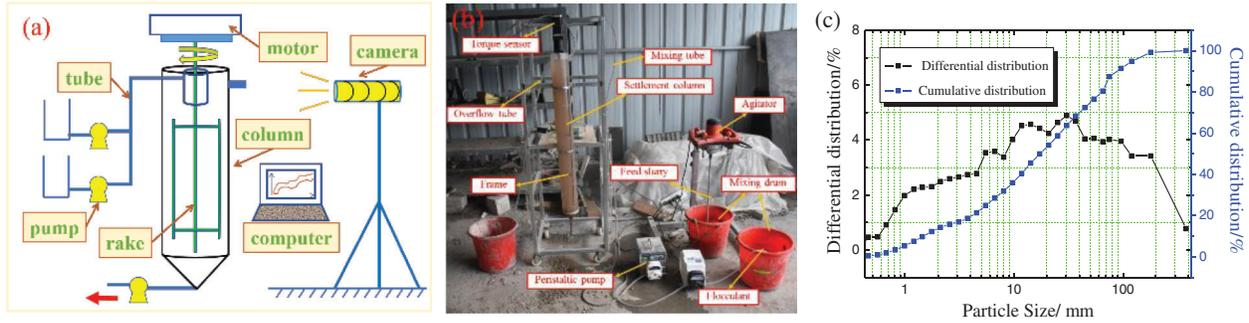
**Figure 1:** The pilot scale continuous thickening test (a) Schematic of thickener (b) Equipments layout (c) Tailings particle size distribution
