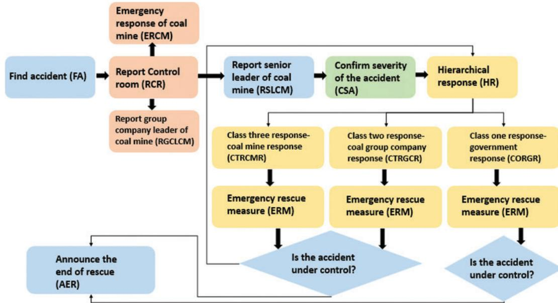
Figure 13: Simplified gas explosion accidents (GEA) emergency rescue workflow of a large coal mine
