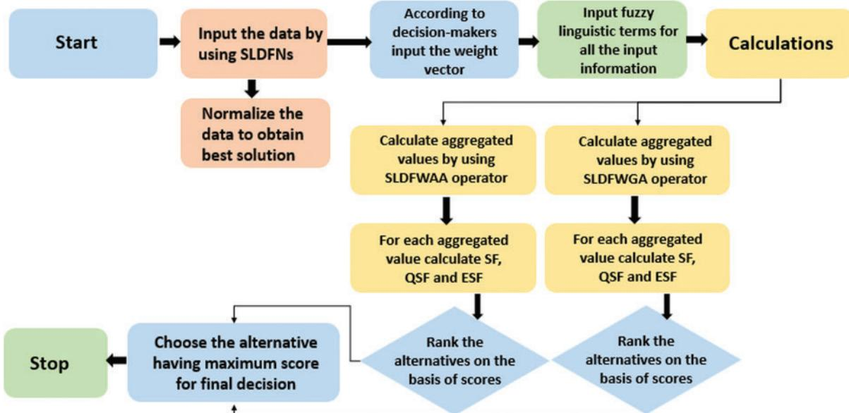
Figure 14: Diagram of the flow map of planned algorithm
