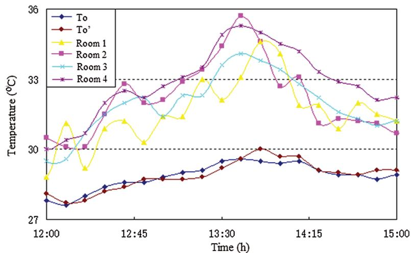
**Figure 5:** The difference between outdoor air temperature and air temperature inside DTHs
