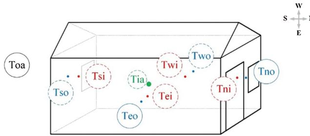
**Figure 3:** Distribution of T-type thermocouple probes in DTH
