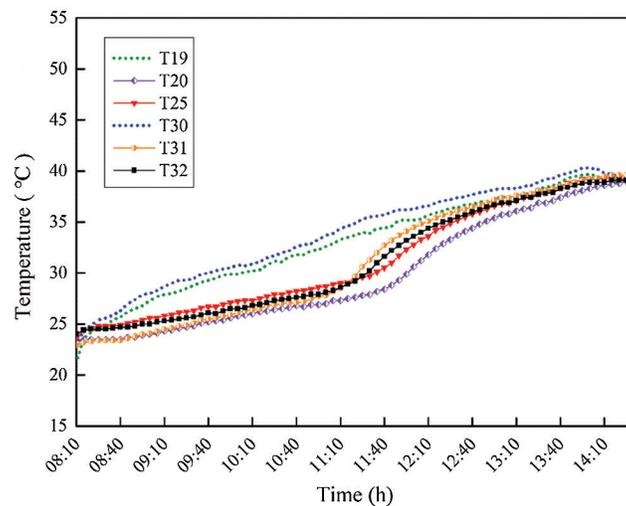
**Figure 11:** Temperature profiles of PCMs and indoor air (Position 3: With distance of 5 mm)
