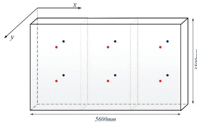
**Figure 4:** Distribution of T-type thermocouple probes in PAS
