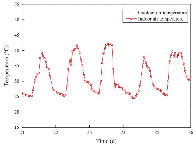
**Figure 7:** Comparison of outdoor air temperature and air temperature inside DTH in summer
