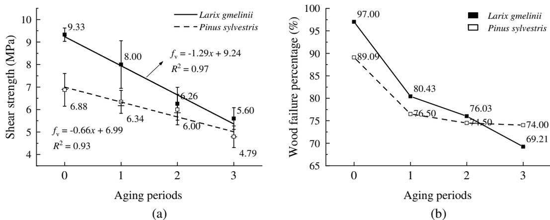
**Figure 6:** Shearing strength of specimens after the accelerated aging process (a) Shear strength of the adhesive layer (b) Wood failure percentage
