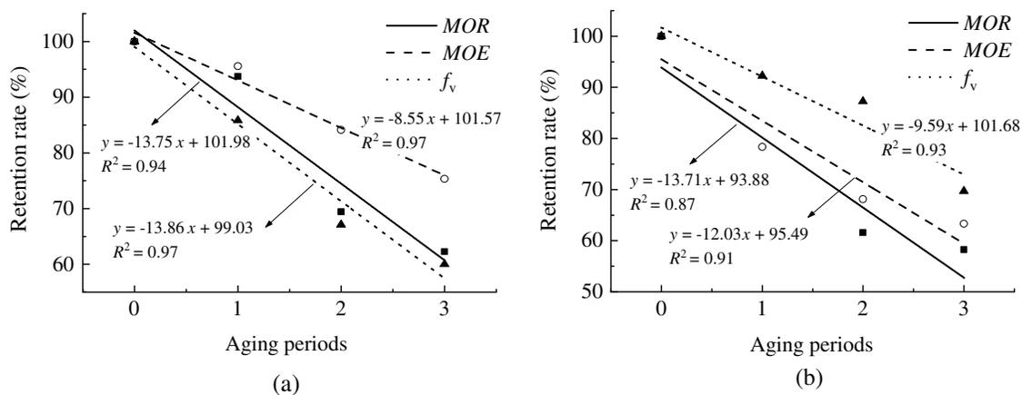
**Figure 7:** Performance changes of specimens after freeze-thaw cycles aging treatment (a) *Larix gmelinii* specimens (b) *Pinus sylvestris* specimens
