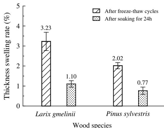
**Figure 4:** Comparison of the thickness swelling rate of different wood species after freeze-thaw cycles and after immersion in water for 24 h
