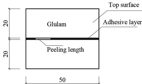
**Figure 2:** Peeling specimen size (all dimensions are in mm)
