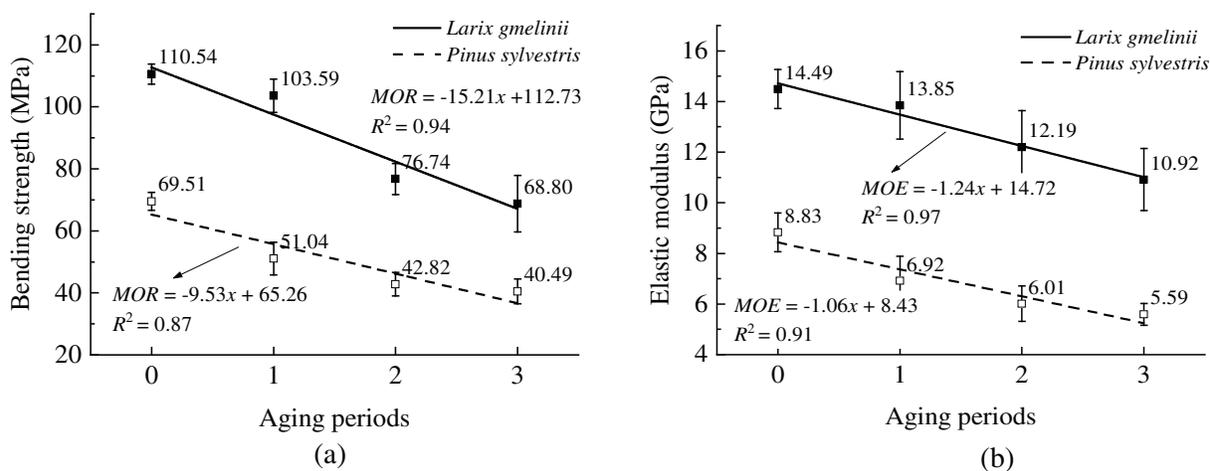
**Figure 5:** Static bending strength and elastic modulus after freeze-thaw cycles aging treatment (a) Static bending strength (b) Elastic modulus
