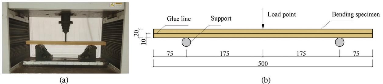
**Figure 1:** Three-point bending test arrangement and specimen size (all dimensions are in mm) (a) Set up used for bending test (b) Specimen size
