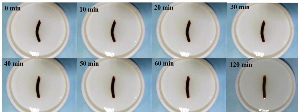
**Figure 7:** The shape recovery behaviors of mono-complex C1D1&Fe hydrogel in 0.1 M EDTA solution at different time
