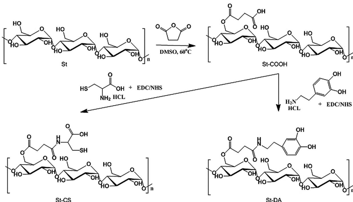
Figure 1: The process to prepare St-CS and St-DA
