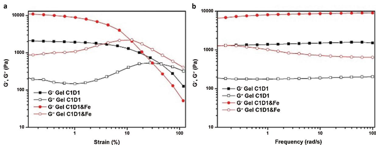
**Figure 4:** The Gel-C1D1 and Gel-C1D1&Fe's stress-strain and stress-frequency curve
