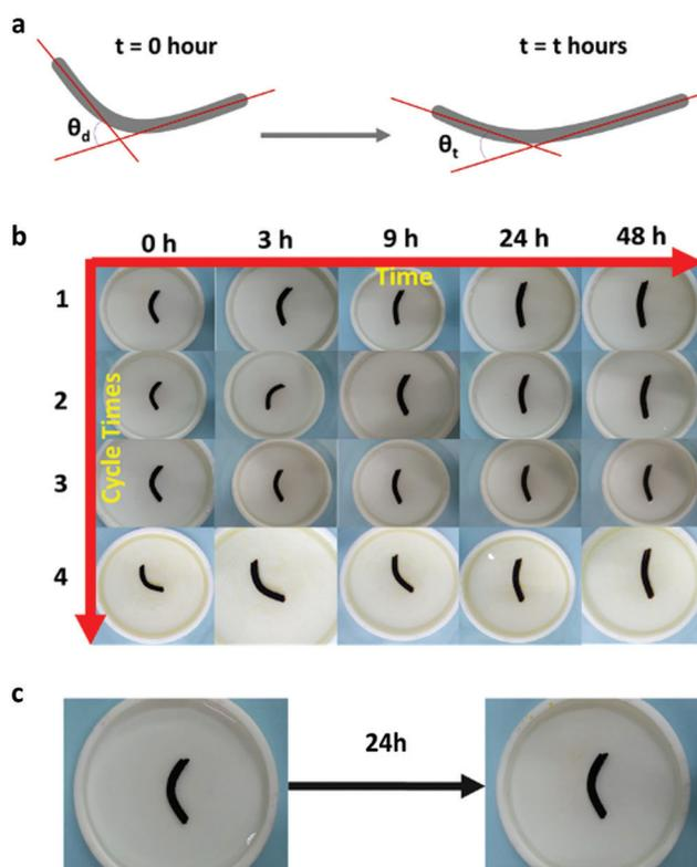
**Figure 5:** a) The angle change at different time; b) The Gel-C1D1&Fe's cycle shape recovery behaviours at different time in pH = 2.0 Tris-HCL buffer solution; c) The Gel-C1D1&Fe's shape recovery behaviours after 24 h in pH = 11 Tris-HCL buffer solution
