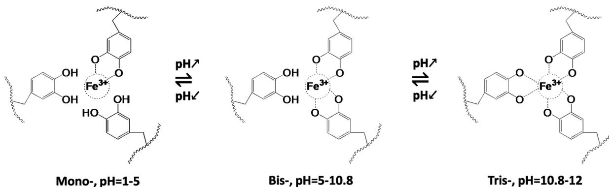
**Figure 6:** The relationship between  $\text{Fe}^{3+}$  and catechol at different pH conditions
