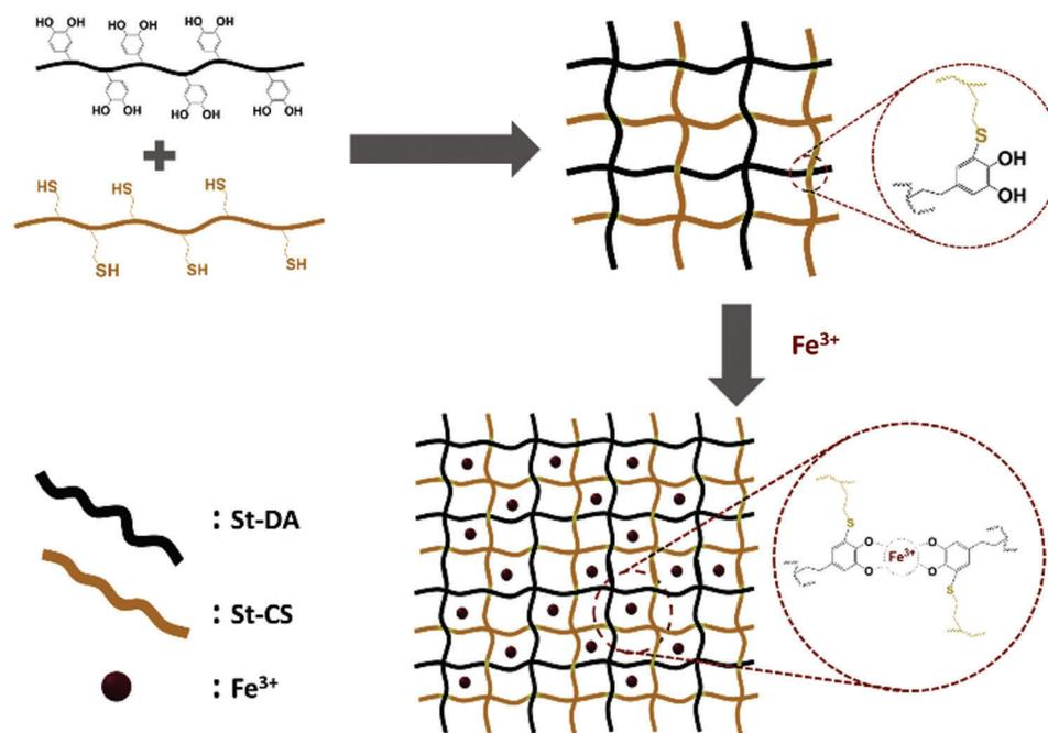
**Figure 3:** The process to prepare the hydrogel with or without Fe<sup>3+</sup> ions
