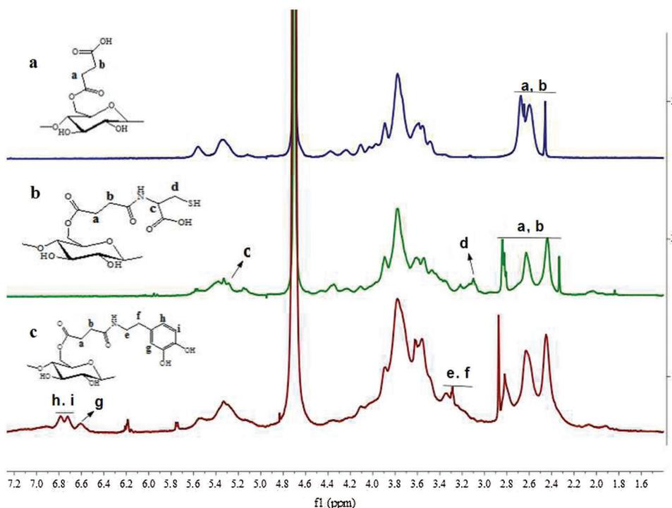
**Figure 2:** The  $^1\text{H-NMR}$  ( $\text{D}_2\text{O}$ ) of St-COOH (a), St-CS (b) and St-DA (c)
