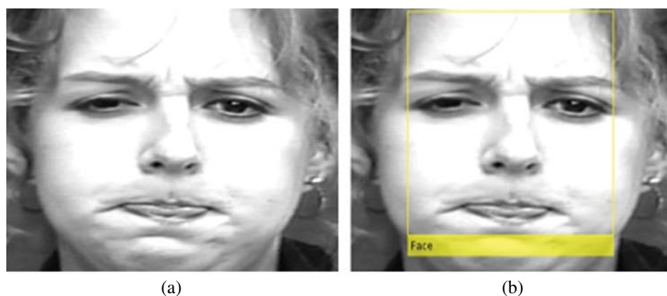
Figure 2: (a) Input image (b) face detection using Viola Jones algorithm
