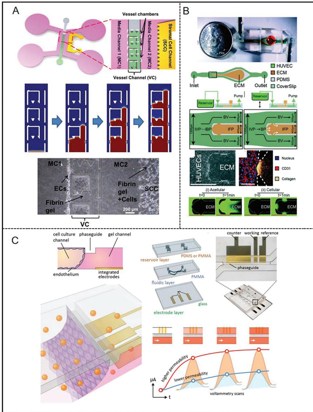
**FIGURE 2.** Examples of microfluidic vascular system for endothelial permeability developed by (A) Lee *et al.* (2014), (B) Akbari *et al.* (2018), (C) Jin *et al.* (2020).
