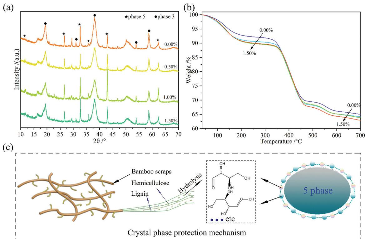
**Figure 6:** Material characterization. XRD diffraction pattern of BR/MO composites (a), TGA curves of composites (b), and crystal protection mechanism (c)
