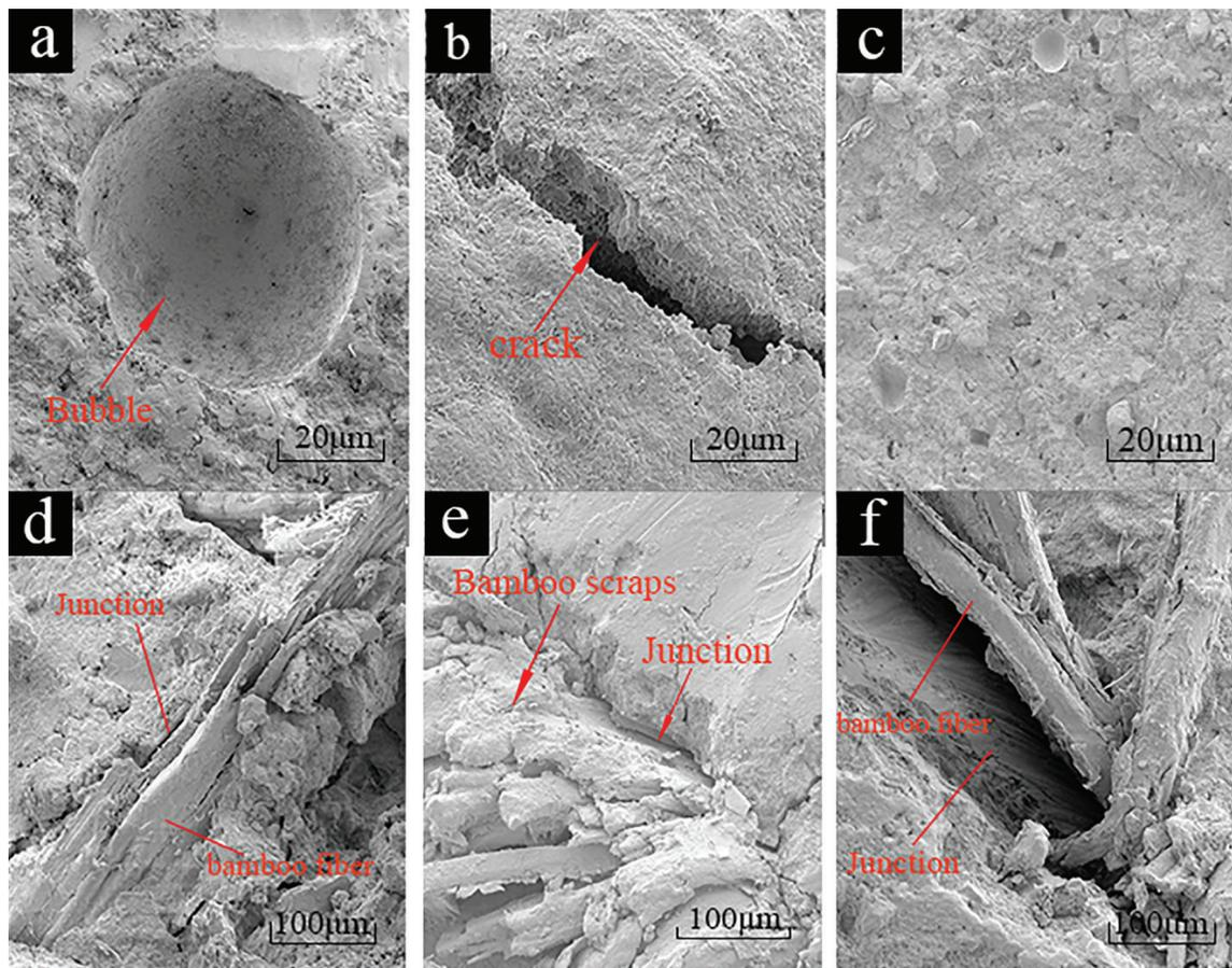
**Figure 5:** Electron micrograph of a composite surface. Surface of MO without BR (a and b); surface of composite with 1.00% BR), with interface between BR and MO (c); bonding interface between BR and MO in composite with 0.50% content (d); bonding interface between BR and MO in composite with 1.00% BR (e); and bonding interface between BR and MO in composite with 1.5% BR (f)
