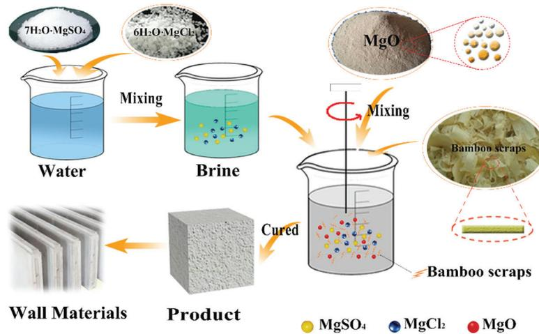
**Figure 1:** Composite material preparation process
