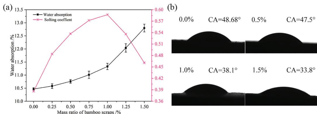
**Figure 4:** Water resistance. Water absorption and softening coefficient of composites with different amount of bamboo scraps (a) and contact angle of composites with different BR content (b)
