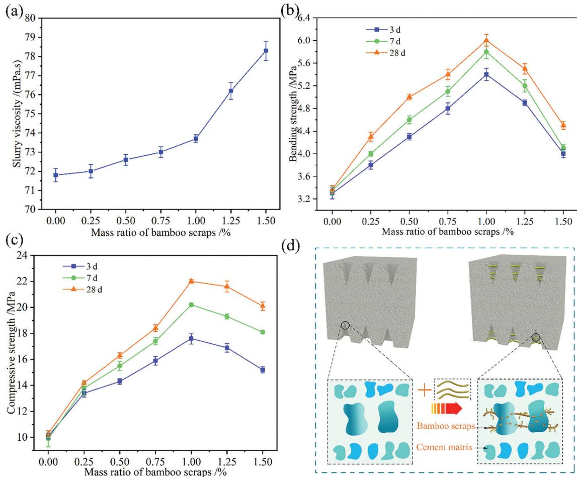
**Figure 3:** Mechanical properties of BR/MO composites. slurry viscosity with different BR content (a), bending strength of composites with different BR content (b), compressive strength of composites with different amount of bamboo scraps (c), and BR mechanism (d)
