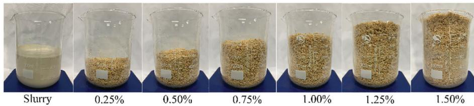
**Figure 2:** Photos of MO slurry and BR for experiments
