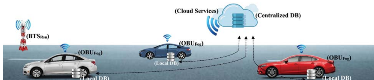
Figure 1: An overview of the IoV architecture, with all nodes equipped with OBUfog and local data repository, connected to a centralized cloud database using BTSRsu
