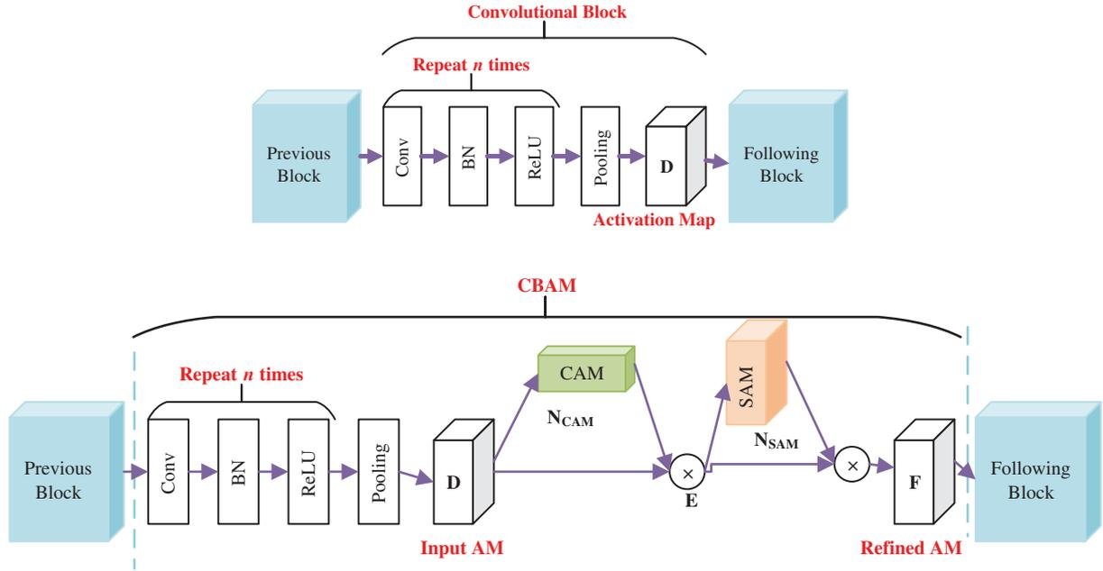
Figure 6: Structural comparison with CB against CBAM. (a) Traditional CB, (b) our CBAM
