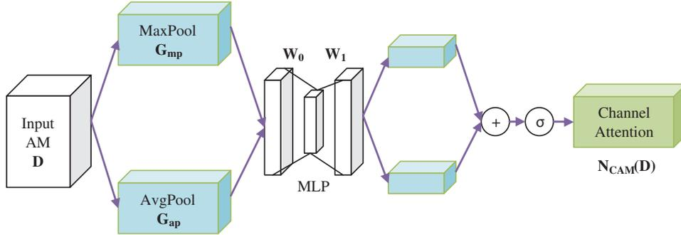
Figure 7: Flowchart of CAM
