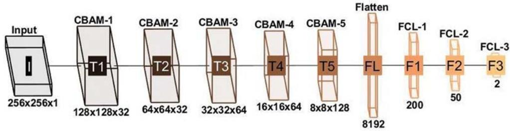
Figure 9: Variables and sizes of AMs of proposed ANC
