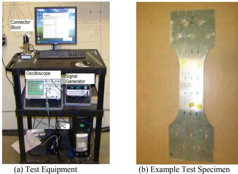
Figure 4: LabVIEW@Controlled Sensor Excitation and Data Collection on Aluminum Test Specimens
