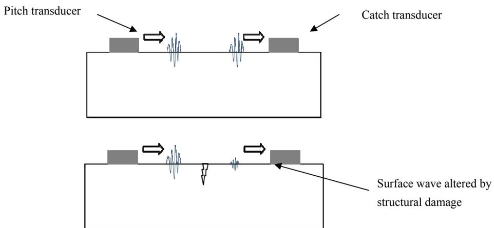
Figure 3: Structural damage causes changes to surface waves detected by guided wave SHM systems
