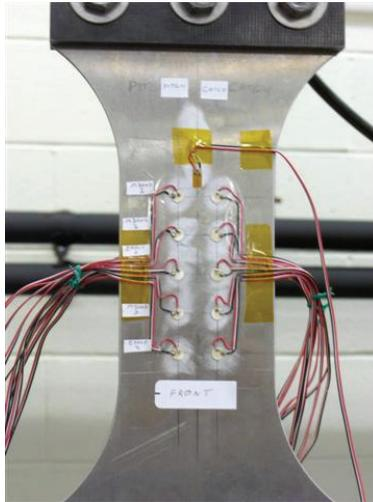
Figure 5: Ten pitch-catch PZT pairs per test specimen, 5 pairs on front, 5 pairs on back (not shown)
