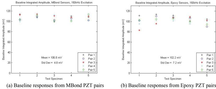
Figure 6: Difference in mean baseline responses from MBond and Epoxy PZT pairs was statistically significant
