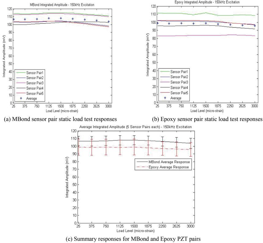
Figure 7: MBond and Epoxy pairs PZT pairs showed no statistical change
