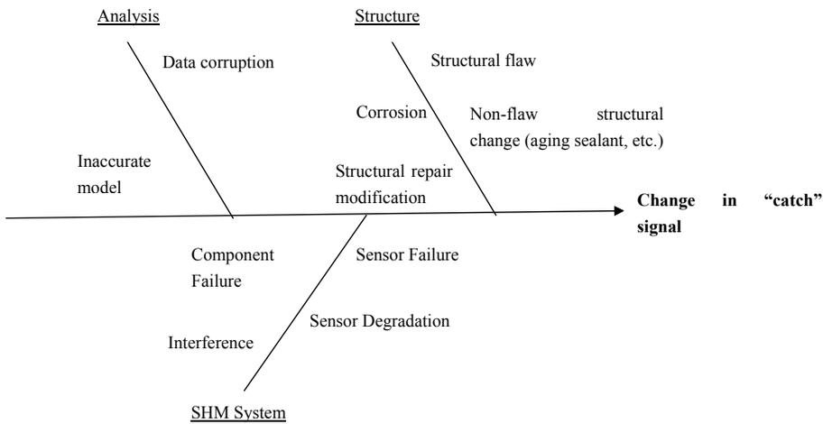
Figure 1: Changes in sensor signals can result from a wide range of factors
