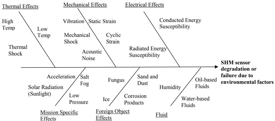
Figure 2: Aircraft environmental factors potentially affecting SHM sensor performance
