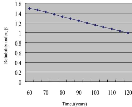
Figure 8: Relationship between reliability index of load-carrying capacity service life and time for Chorng-ching viaduct.
