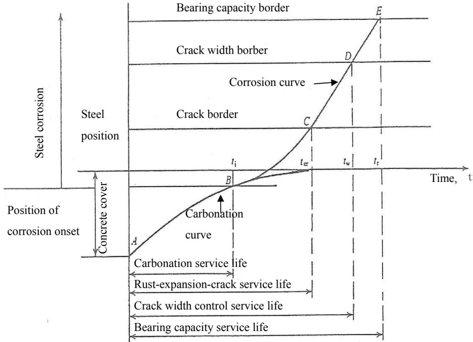
Figure 1: Schematic diagram of steel corrosion and service life of reinforced concrete structures.
