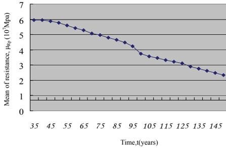
Figure 9: Relationship between mean of resistance and time for Wann-fwu bridge.
