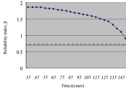
Figure 6: Relationship between reliability index of load-carrying capacity service-life and time for Wann-fwu bridge.
