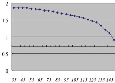
Figure 5: Relationship between durability degree of load-carrying capacity service life and time for Wann-fwu bridge.
