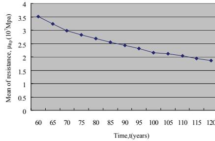
Figure 10: Relationship between mean of resistance and time for Chorng-ching viaduct.
