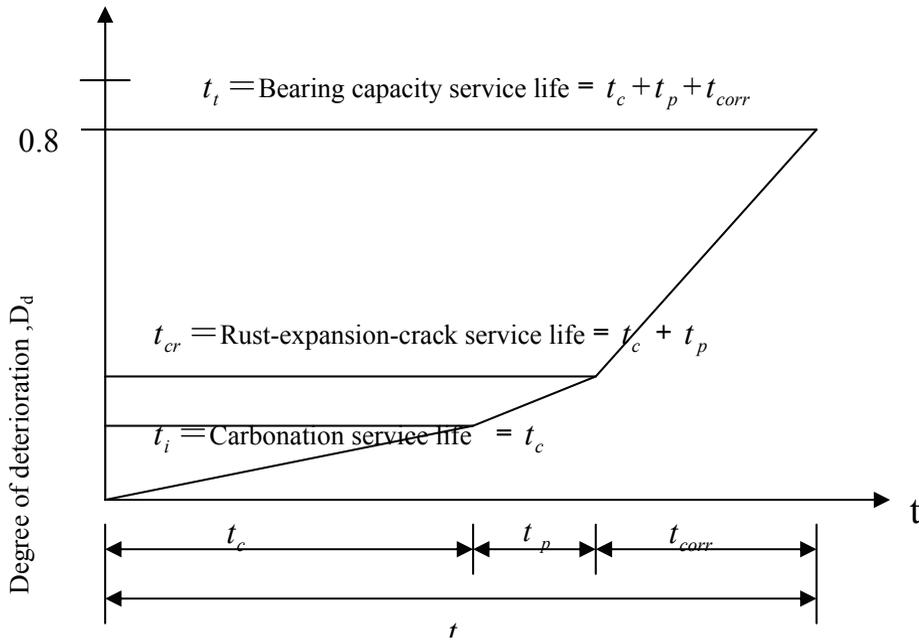
Figure 2: Schematic diagram of service life of existing reinforced concrete bridges.
