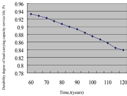
Figure 7: Relationship between durability degree of load-carrying capacity service life and time for Chorng-ching viaduct.
