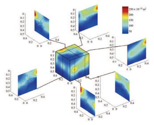
Figure 1: The permeability inhomogeneity in the cuboidal block of Indiana Limestone [Selvadurai and Selvadurai, 2010]
