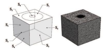
Figure 2: The sub-cube model of the porous medium with the annular permeameter. [Selvadurai and Selvadurai, 2010]
