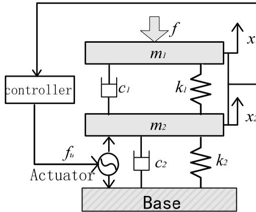
Figure 1: Double-layer Vibration Isolation System
