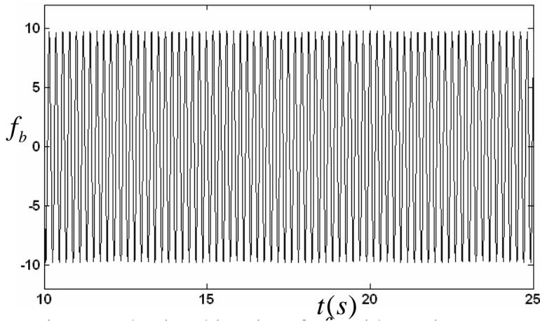
Figure 6: The time histories of  $f_b$  with passive system
