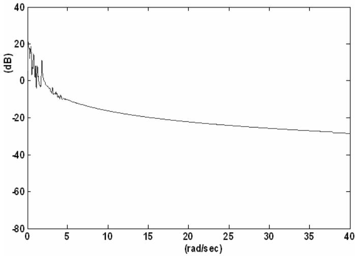
Figure 8: The power spectrum of  $f_b$  with chaos synchronization
