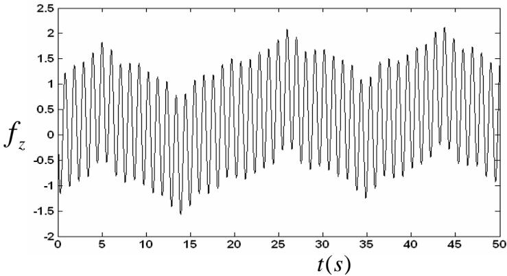
Figure 9: The time histories of force passed to base with chaos synchronization
