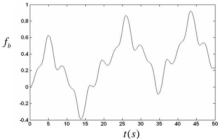
Figure 7: The time histories of  $f_b$  with chaos synchronization
