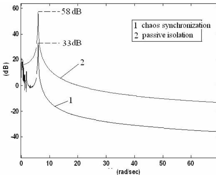
Figure 11: The power spectrum of fore passed to base
