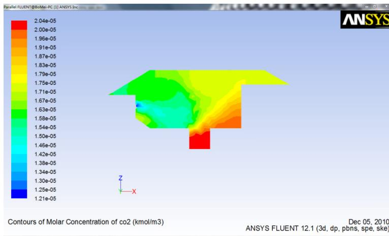
Figure 11: Concentration of Carbon Dioxide (Case 4)
