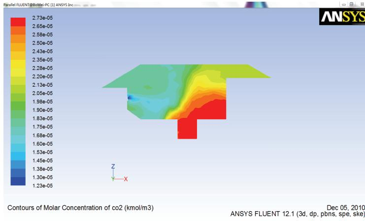
Figure 10: Concentration of Carbon Dioxide (Case 3)
