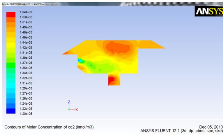
Figure 4: Concentration of Carbon Dioxide (Case 6)
