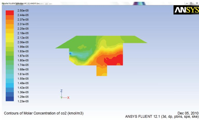
Figure 9: Concentration of Carbon Dioxide (Case 2)
