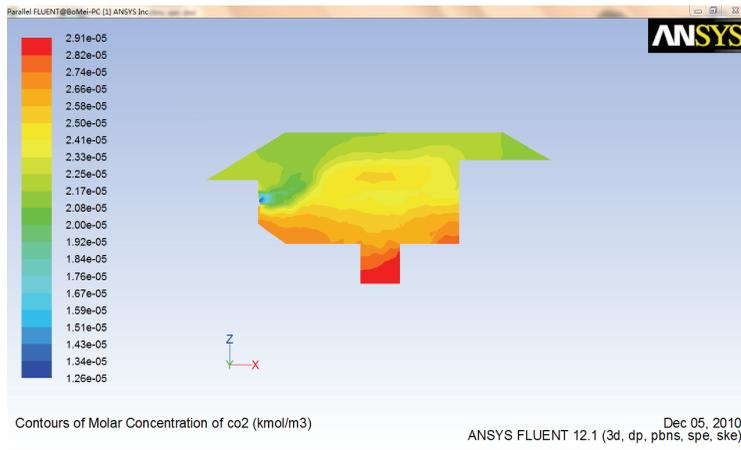
Figure 8: Concentration of Carbon Dioxide (Case 1)
