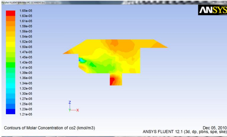
Figure 12: Concentration of Carbon Dioxide (Case 5)
