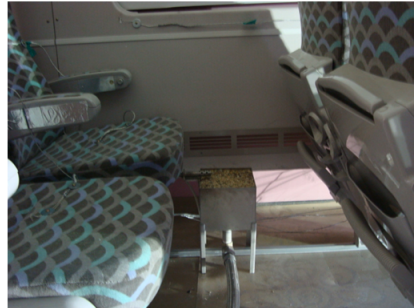
Figure 3: Sand burner installed between seats
