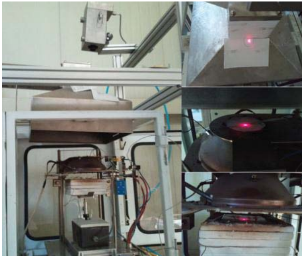
Figure 1: Pyrometer install and measurement range of pyrometer at each position
