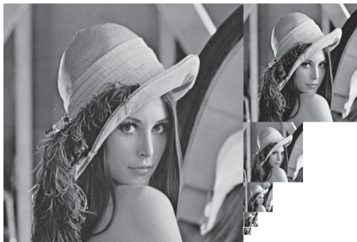
Figure 3: Example of Gaussian Pyramids
