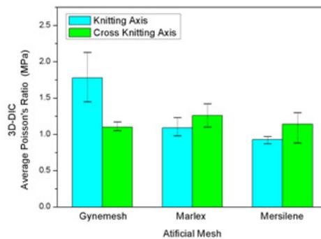
Figure 8: The histogram of average Poisson's ratio obtained from the 3D-DIC method
