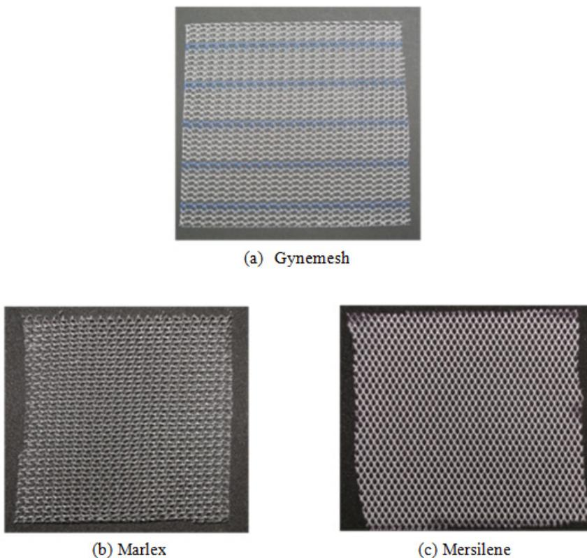
Figure 3: Photographs of the three types of artificial mesh.
