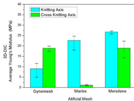
Figure 7: The histogram of average Young's modulus obtained from the 3D-DIC method.
