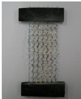
Figure 5: The artificial mesh after spraying the speckles. Rubber end tabs were adhered onto the two ends of the test specimen
