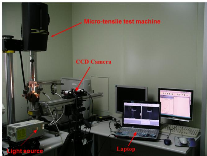
Figure 4: Photograph of the tensile test setup with the VIC-3D system.
