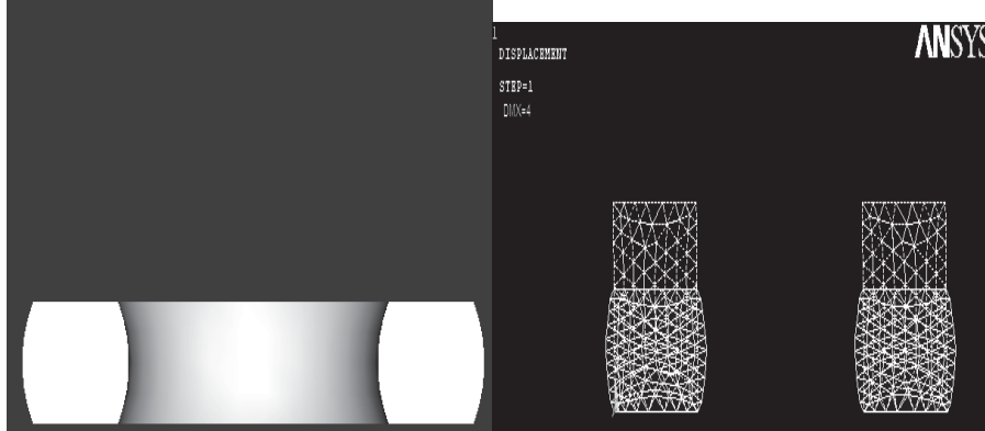
c) Deformation of physical model at 450k d) Deformation of FE Modelat 473k
