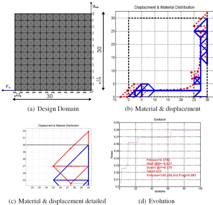
Figure 3: Results: 12x12 subcells, Volume fraction: 8.3% (3x3 : 30%)
