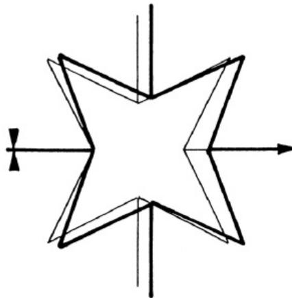
Figure 1: Star shaped, two dimensional representative cell made of beams and deformed shape indication an auxetic homogeneous.
