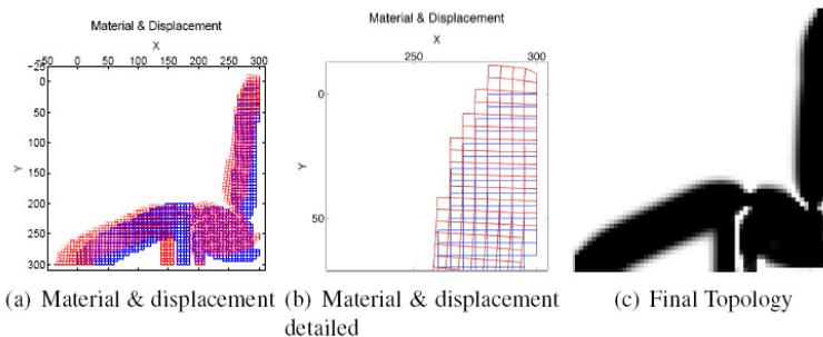
Figure 5: A resulted topology for a 60x60 design domain, with Volume goal at 30%
