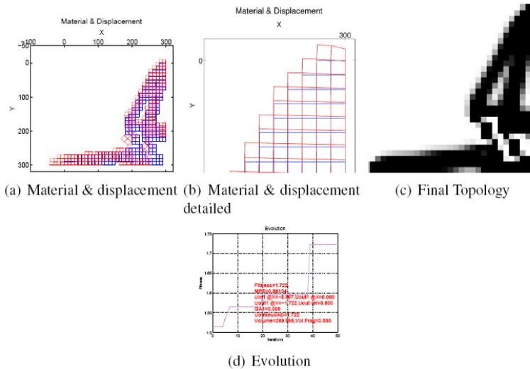
Figure 4: A resulted topology for a 30x30 design domain, with Volume goal at 30%
