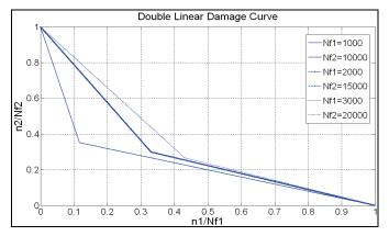
Figure 3: Double Linear Damage Curve Approach
