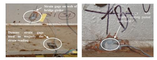
Figure 8: Typical arrangement of strain gages on the flange and the web of the plate girder
