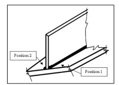
Figure 10: Locations of the strain gages at the welded section
