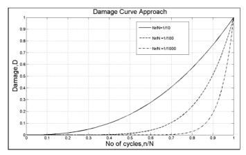
Figure 4: Damage curve approach
