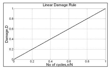
Figure 1: Linear damage rule (LDR)
