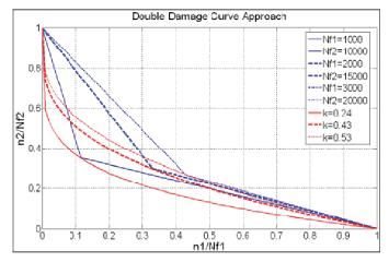
Figure 5: Double Damage Curve Approach
