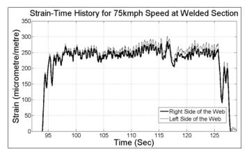
Figure 11: Strain-time history on weld section of flange plate
