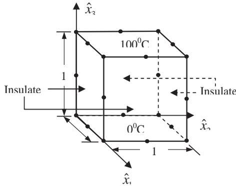
Figure 1: A unit cube with a temperature gradient – Example I
