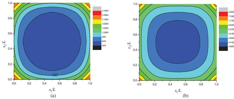
Figure 3: Contour plots of normalized von Mises equivalent stresses of the transversely isotropic rectangular column as obtained from the BEM analysis: (a) at the bottom face,  $x_3 = 0$ ; and (b) at the top face,  $x_3 = H$ . (Example II)
