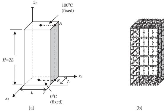
Figure 2: *Example II* - A rectangular column with a thermal load: (a) the physical problem, lateral surfaces thermally insulated, (b) the BEM mesh (216 boundary elements).
