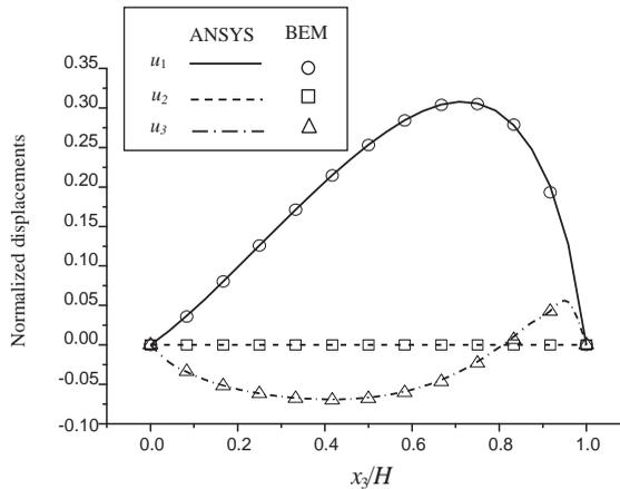
Figure 4: Variations of the normalized displacements along the line  $AB$  on the transversely isotropic rectangular column under thermal load – Example I
