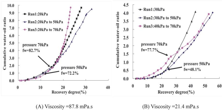
Figure 6: The effort of changing drawdown pressures on the variation of cumulative water-oil and recovery at different water cut.
