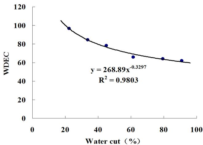
Figure 8: Water driving effective coefficient versus water cut at altering drawdown pressure.
