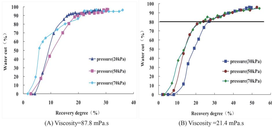
Figure 3: Water-cut raise curves of two oil viscosities under different drawdown pressures.
