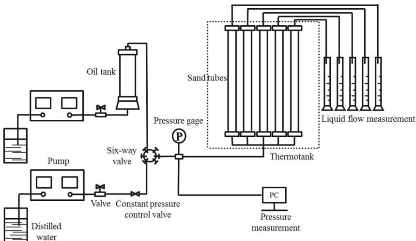
Figure 2: The apparatus diagram of the simulation system.
