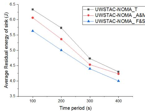
**Figure 3:** Residual energy of sink versus Time period
