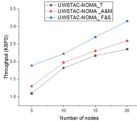
**Figure 2:** Throughput vs. Number of sensors
