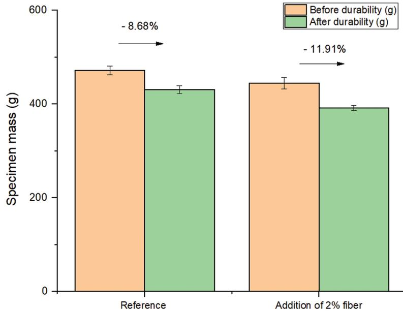
**Figure 8:** Result of loss of mass (g) for wetting and drying cycle
