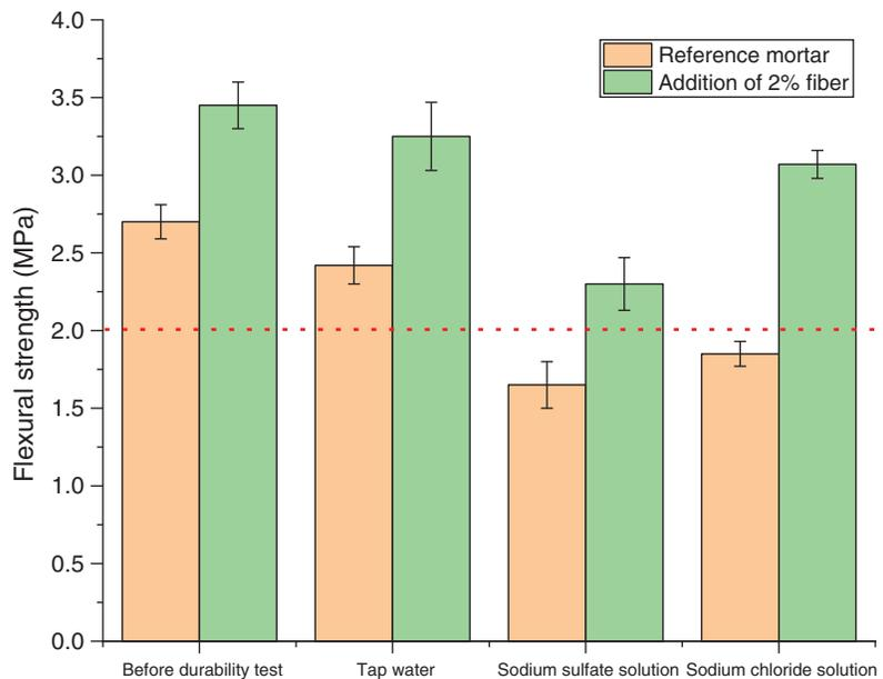
**Figure 5:** Result of the flexural strength (MPa)
