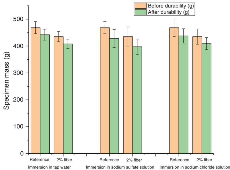
**Figure 3:** Result of loss of mass (g) for attack durability of aggressive agents
