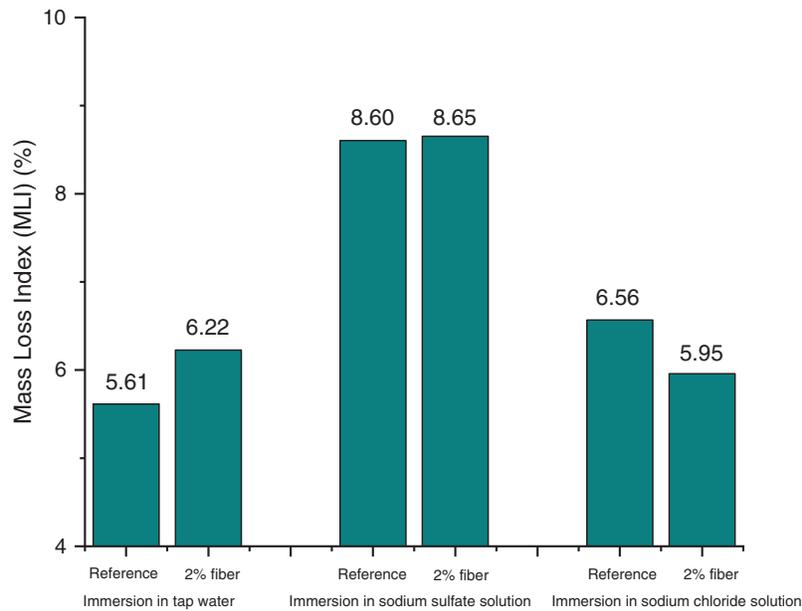
**Figure 4:** Mass loss index (MLI) for specimens
