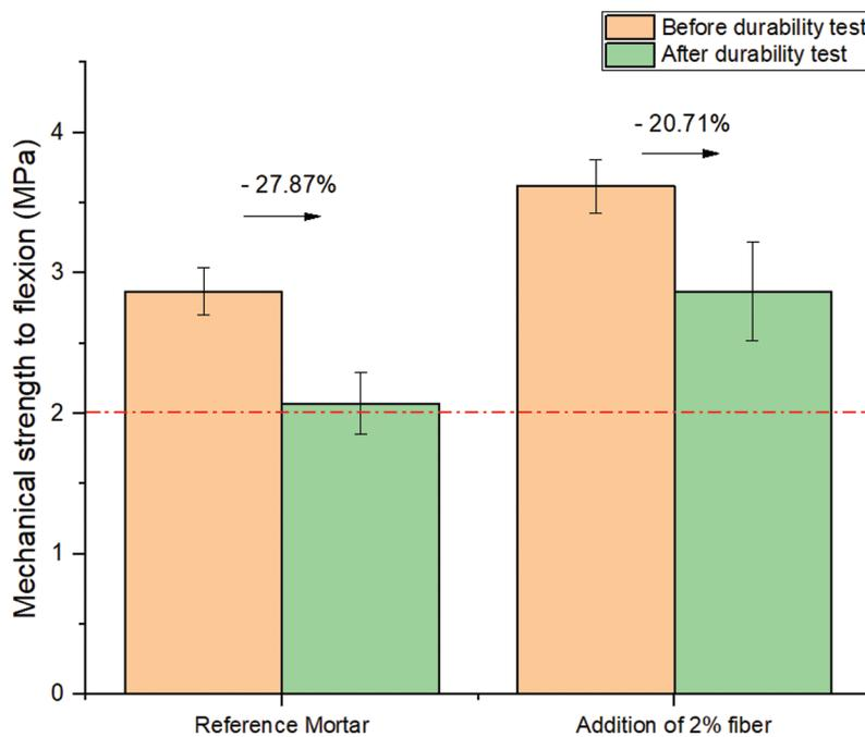
**Figure 9:** Result of flexural strength (MPa) for wetting and drying cycle
