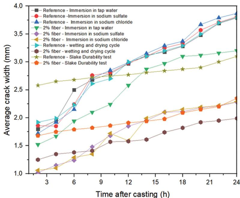
**Figure 11:** Results of the shrinkage cracking tests
