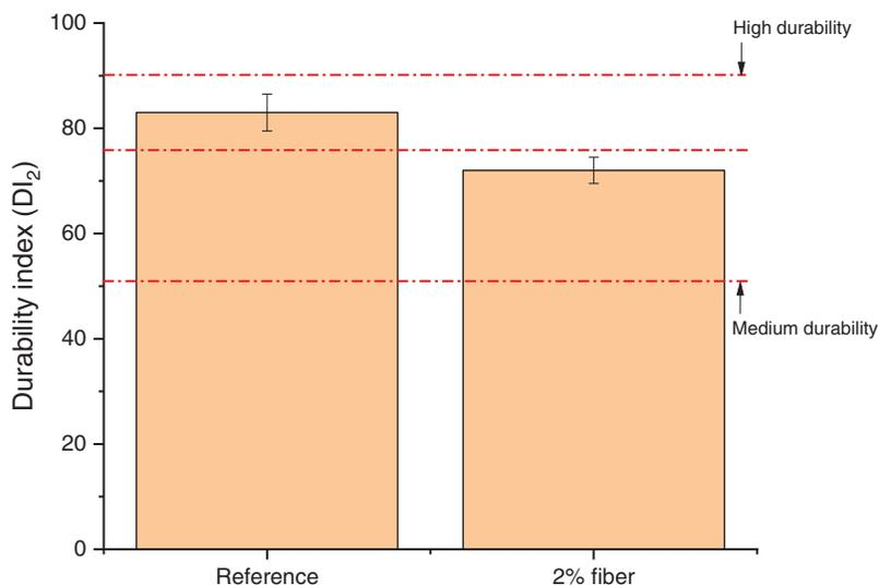
**Figure 10:** Durability index of specimen fragments after slake durability test
