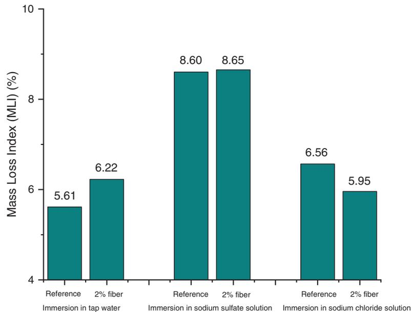
**Figure 4:** Mass loss index (MLI) for specimens
