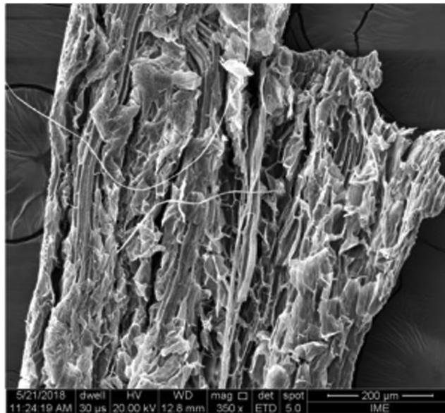
**Figure 2:** SEM of curaua fiber after treatment with NaOH
