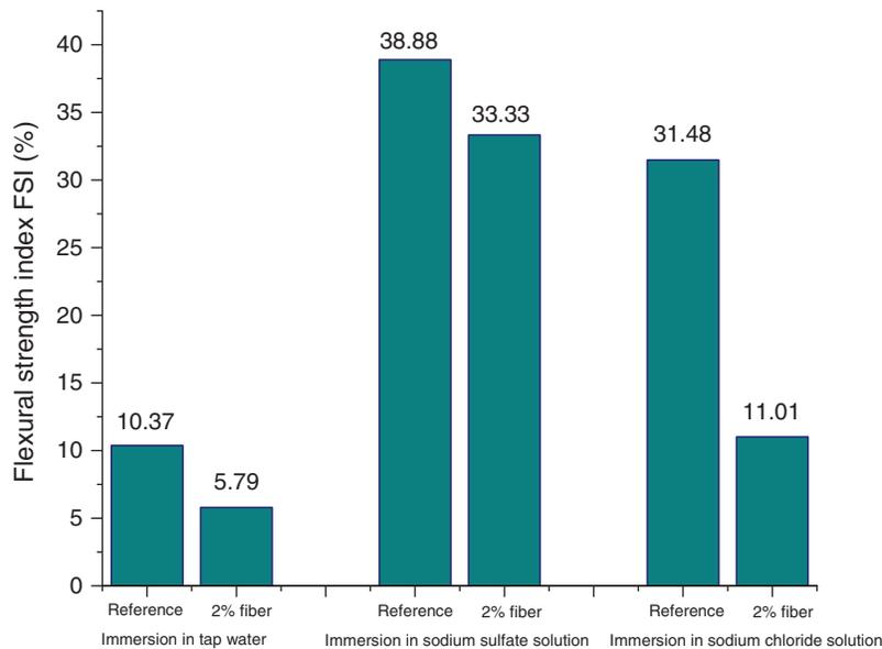
**Figure 6:** Flexural strength index (FSI) for specimens
