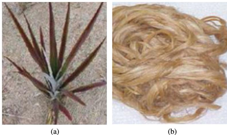
**Figure 1:** Curauá fiber: (a) Curauá plant (b) Natural curauá fiber [27]
