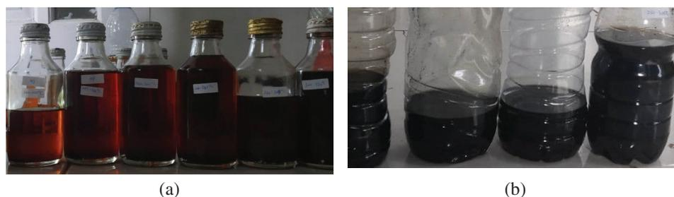
**Figure 3:** LDPE plastic pyrolysis liquid product: (a) without catalyst and (b) with activated natural zeolite catalyst
