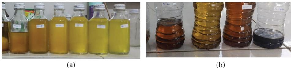
**Figure 2:** PP plastic pyrolysis liquid product: (a) without catalyst and (b) with activated natural zeolite catalyst
