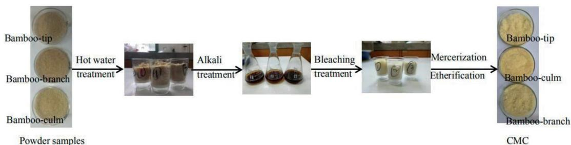
**Figure 2:** The process for preparing CMC from different parts of bamboo powder
