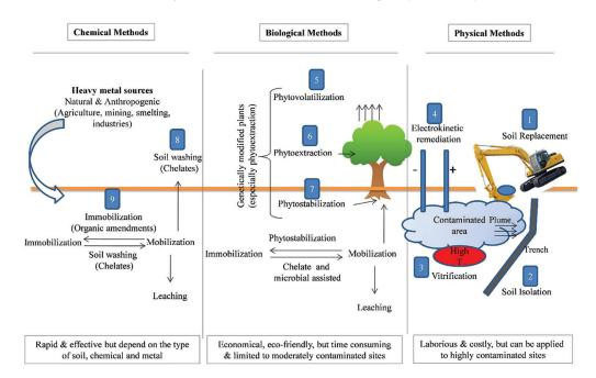
Figure 2: Classification and comparison of remediation methods for heavy metal contaminated soils [23]
