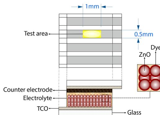
**Figure 1** Scheme of the fabricated solar cells. Effective area of photon conversion:  $0.50 \text{ cm}^2$ .
