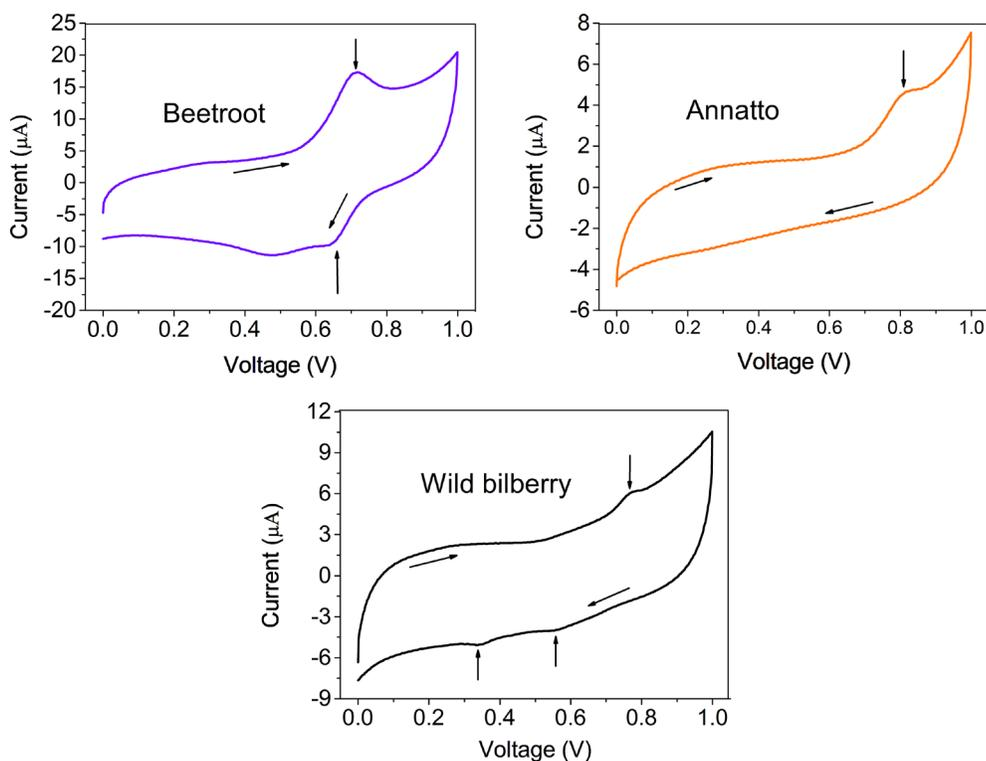
**Figure 8** CV curves for the studied dyes at positive potential (1V/s). These electrochemical measures were referred to as Ag/AgCl, KCl<sub>saturated</sub> electrode. Vertical arrows denote first oxidation couples.
