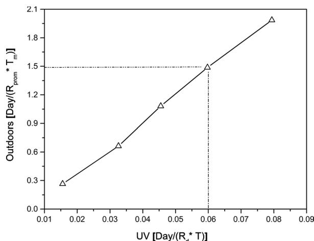
Figure 7 Correlation between UV Chamber and Outdoors measurements, considering radiation and temperature in each exposition media. Curve applies only between 1–4 days at UV Chamber (R2: 0.9970). UV Chamber (Rd = 0.89 W/m<sup>2</sup>\*nm, T = 60°C – Outdoors (Rprom = Rm<sup>a</sup> / 340nm, Tm<sup>a</sup>).<sup>a</sup>Data taken from Table 3.
