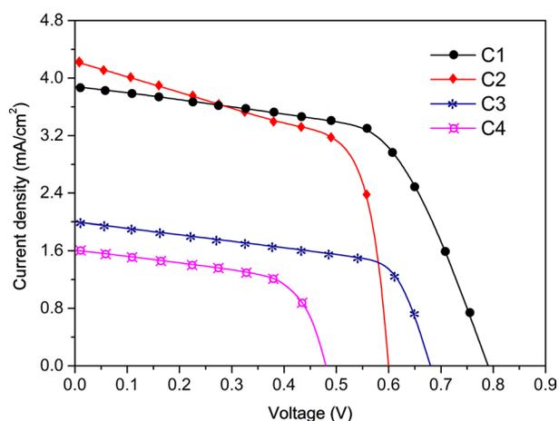
**Figure 12** I-V curves for the fabricated solar devices. Rate scan: 0.05V/s.
