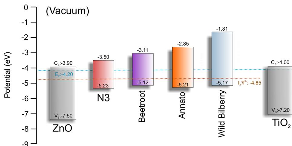
Figure 9 Relation between energetic levels of the studied dyes and conventional semiconductors used in a DSSC architecture.
