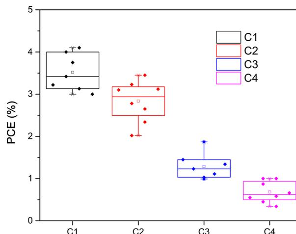
Figure 11 Efficiency of fabricated DSSCs with the obtained natural dyes.
