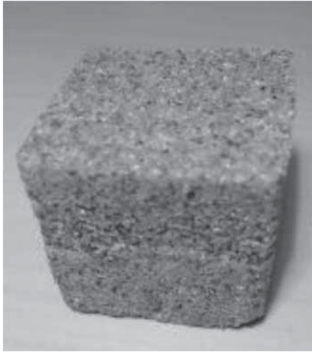
Figure 1 Biocomposite specimen bound with bovine serum albumin (BSA) protein. (Specimen shown is a 25 mm × 25 mm × 25 mm cube.)
