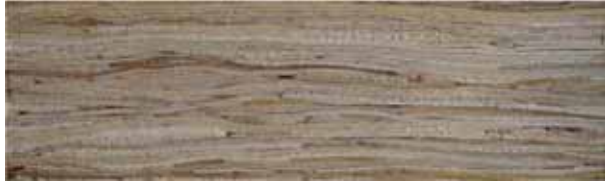
Figure 1 Strand undulations in the longitudinal direction.
