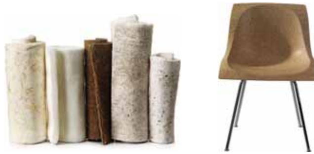
Figure 4 Industrially produced nonwoven mats from cellulose and bark (left) used for the Imprint chair (right) by Johannes Foersom, Peter Hiort-Lorenzen launched in 2005. The mats were designed carefully for desired surface properties.
