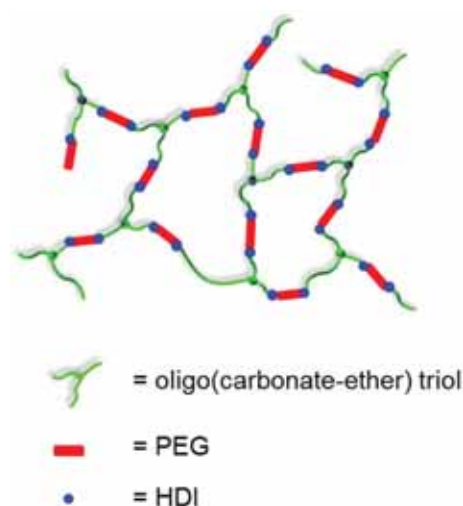
Scheme 2 Schematic diagram of the structure of the Triol-PEG networks.
